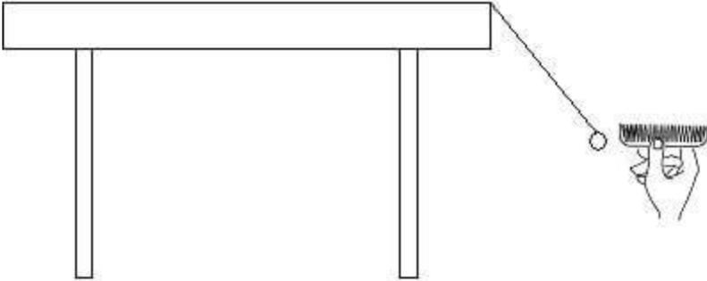
Figure 2. The activity setup for using static electricity to attract an O-shaped cereal with a comb.
